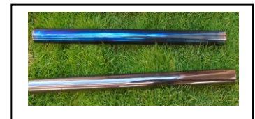
Image of single and two layer tandem absorber tubes developed by a cost effective process
